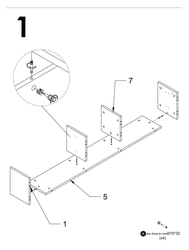
1. Assemble the top panel and bottom panel.
