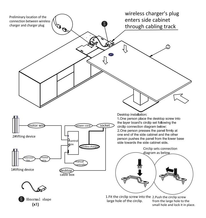
1. Raise the desktop and use screws to fix the side cable box;
