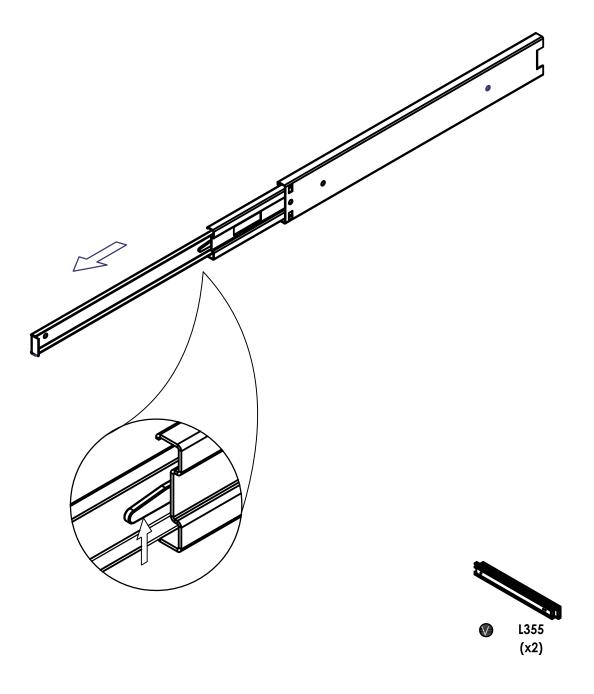
1.Install the 3-stage sliding rail on the cabinet;
