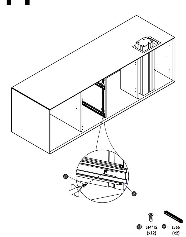
1.Install the 3-stage sliding rail on the drawer;
