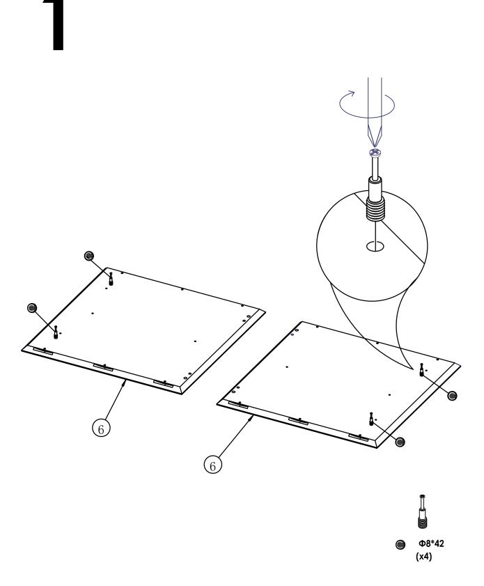
1.Install Cam lock on the side cabinet bottom layer board #5;
