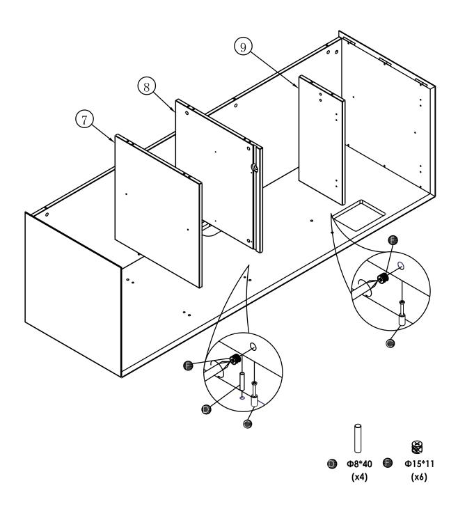
1.Install cam lock on the side cabinet top layer board#11;
