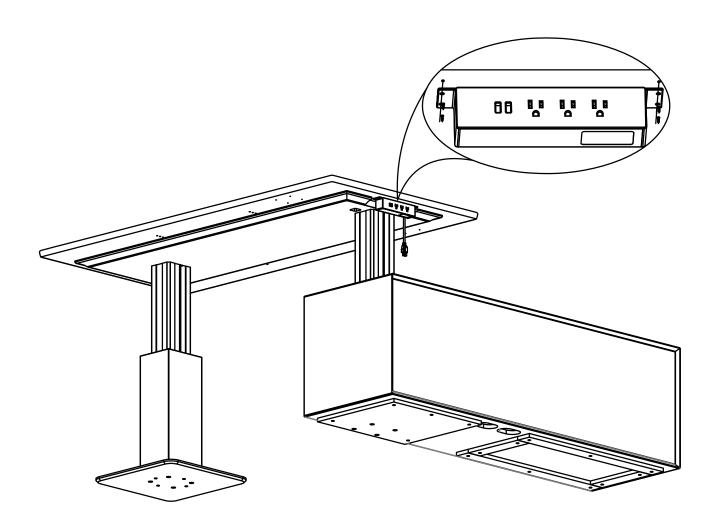
1.Install square shape coiled tube, put the cable plug and cable wires to side cabinet inside from the square hole;
