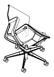
2. Adjust tension controller n the initial horizontal state, pull the left wire control handle outward to unlock, and continue to pull the handle outward to lock.
