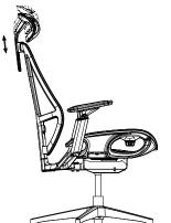
2. Armrest function and seat back up and down adjustment
