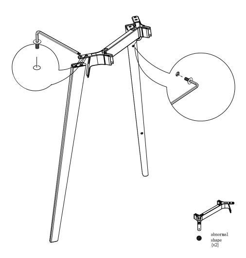
1. Remove the pre-installed 8 M8\*16 screws inside the leg connectors.
