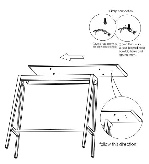
1. Install the shielding piece on the tabletop.
