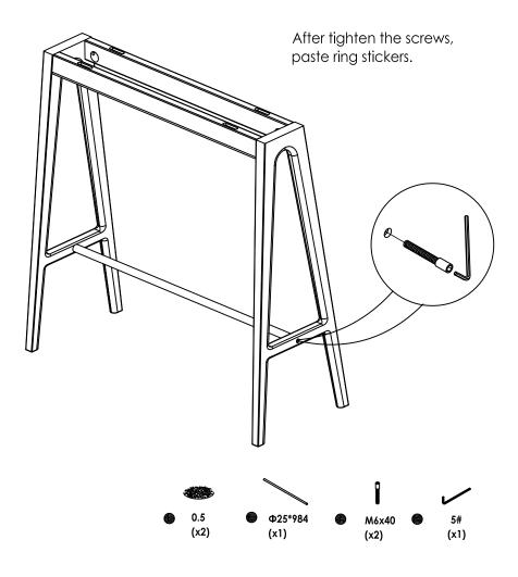
1. Install the circlip strews on the tabletop.
