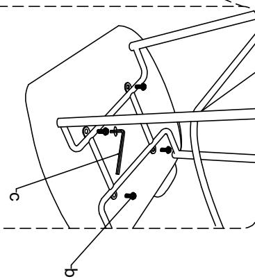
Use 4 Allen screws (M8\*20) to connect the steel feet with the seat cushion and fix it
